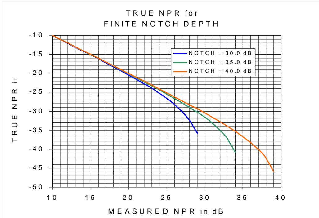
**Figure 3. Correction chart for true NPR for finite notch depth**
